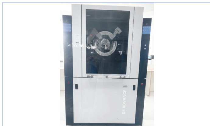
[Table/Fig-4]: X-ray diffractometer (Bruker D8 Advance) used for crystalline structure analysis of Morin-mediated nanoparticles.
