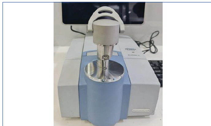
[Table/Fig-2]: Fourier Transform Infrared (FTIR) Spectrophotometer (Bruker Alpha II) used for characterisation of Morin-mediated nanoparticles.
