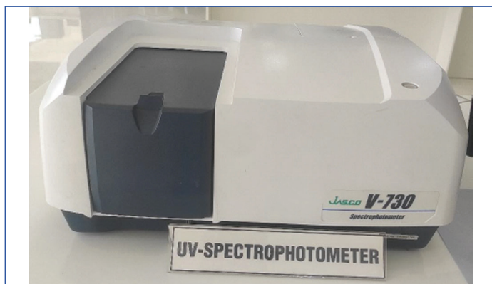
[Table/Fig-3]: UV-Visible Spectrophotometer (JASCO V-730) used for optical characterisation of Morin-mediated nanoparticles.
